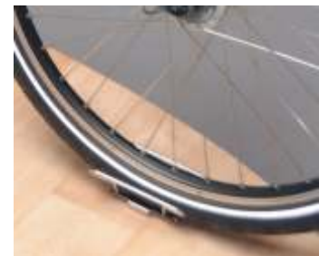
Detailed view: the bicycle is held in a straight line with Big-Wheel Clips.
